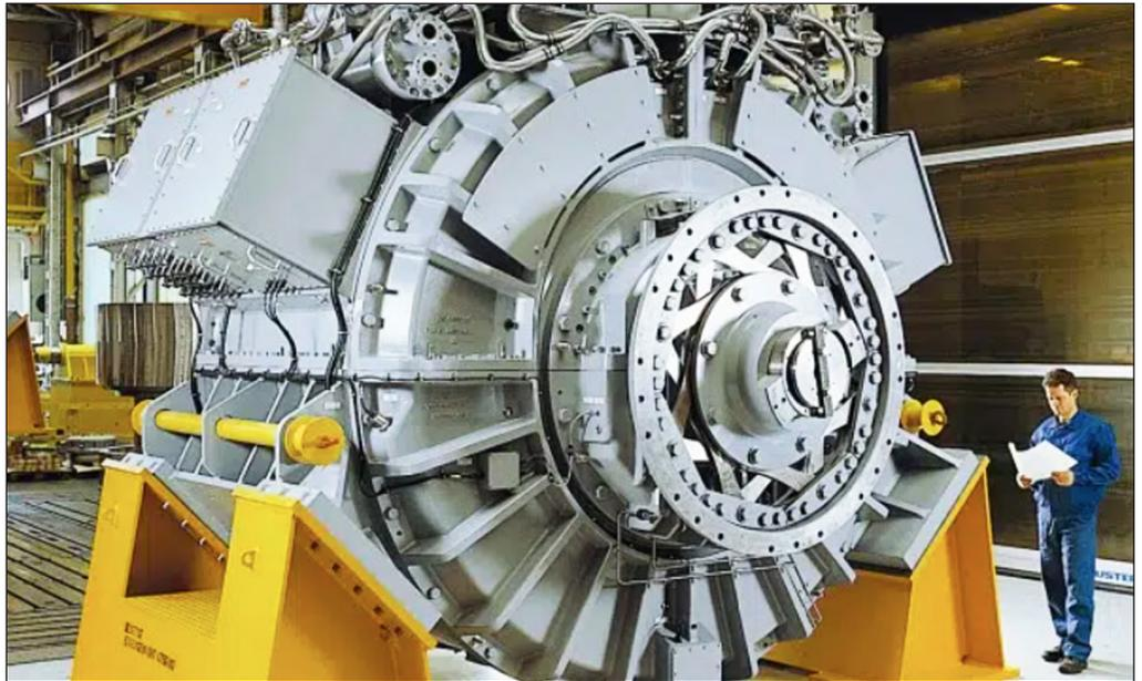
Siemens Permasyn motor for submarines. (Siemens photo.)
